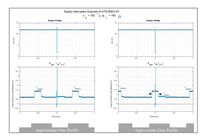
Figure 13: Example of ATS19581 continued operation in presence of 20  $\mu$ s supply voltage interruption (a) at left, supply interruption with output in  $I_{CC(LOW)}$  (b) at right, supply interruption with output in  $I_{CC(HIGH)}$
