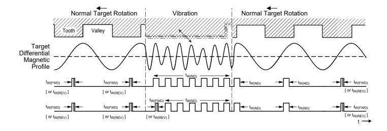
Figure 9: Output protocol options with non-direction pulses
