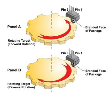
Figure 6: Target Rotation ("F" Variant Shown)
