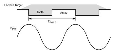
Target Cycle; the amount of rotation that moves one tooth and valley across the sensor.
