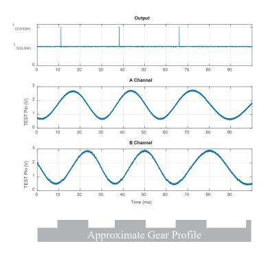
Figure 11: Example TEST Pin Signals
