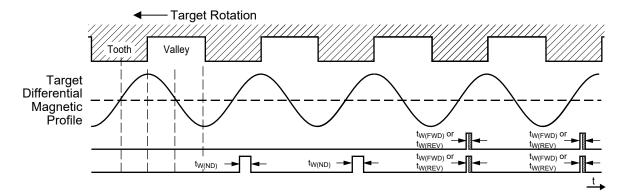
Figure 7: Output options after power-on ("-FS" or "-RS")
