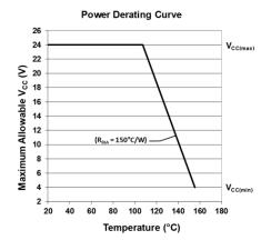
A worst-case estimate,  $P_{D(max)}$ , represents the maximum allowable power level ( $V_{CC(max)}$ ,  $I_{CC(max)}$ ), without exceeding  $T_{J(max)}$ , at a selected  $R_{\theta JA}$  and  $T_A$
