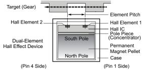
Figure 1: Relative Motion of the Target
