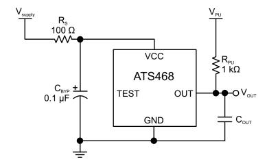
**Figure 6: Typical Application Diagram**
