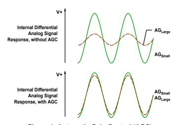
Figure 4: Automatic Gain Control (AGC)
