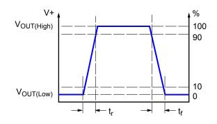
Figure 2. Output Rise Time and Output Fall Time
