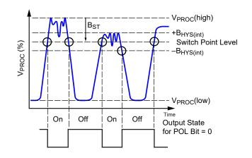
Figure 7. Switching on internal hysteresis
