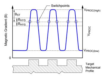
Figure 4. Running Mode Switch Point and Internal Hysteresis
