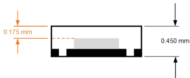
Figure 18: XtremeSense TMR Sensor Location in z Dimension for CT310 in DFN-8 Package
