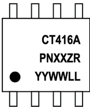
Figure 14: CT416 Device Marking for 8-Lead Package
