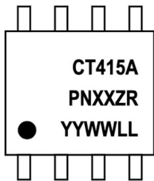
Figure 15: CT415 Device Marking for 8-lead Package
