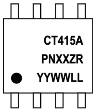
Figure 22: CT415 Device Marking for 8-lead Package
