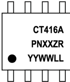
Figure 44: CT416 Device Marking for 8-lead Package
