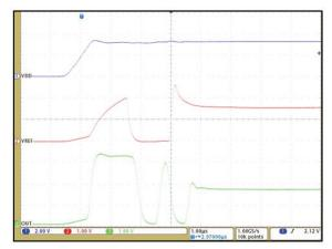
Figure 5: CT416 Startup Waveforms for V<sub>OQ</sub> = 1.65 V (AC Current)
