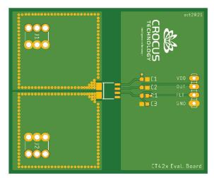
Figure 16: Recommended PCB Layout (Top Layer) for the 20 A to 65 A variants of the CT416
