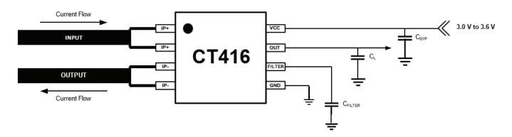
Figure 2: CT416 Application Block Diagram
