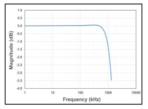
Figure 7: CT416 Bandwidth with  $C_{FILTER} = 1.0 pF$
