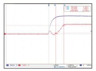
Figure 9: CT416 Rise Time;  $I_p = 30 A_{PK}$  and  $C_L = 100 pF$
