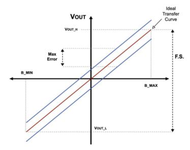
Figure 13: Total Output Error (EOUT) vs. Sensed Current (IP)
