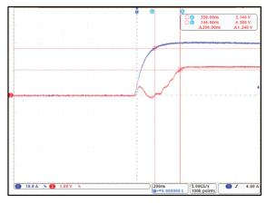
Figure 8: CT416 Response Time;  $I_P = 30 A_{PK}$ and  $C_L = 100 pF$
