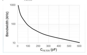
Figure 12: Experimental Bandwidth vs.  $C_{FILTER}$ Sensitivity
