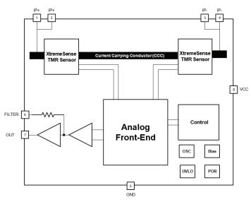
Figure 1: CT416 Functional Block Diagram for 8-lead SOIC Package
