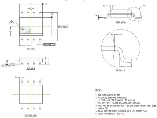
Figure 19: SOIC-8 Package Drawing and Dimensions
