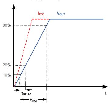
Figure 15: CT416 Propagation Delay and Rise Time Curve
