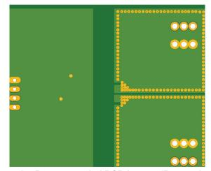
Figure 17: Recommended PCB Layout (Bottom Layer) for the 20 A to 65 A variants of the CT416
