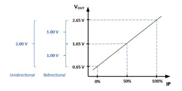
Figure 11: Linear Output Voltage Range (OUT) vs.
