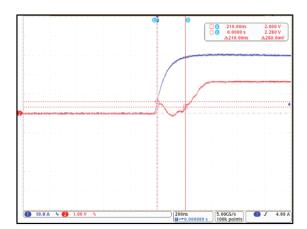
Figure 10: CT416 Propagation Delay;  $I_P$  = 30  $A_{PK}$  and  $C_L$  = 100 pF
