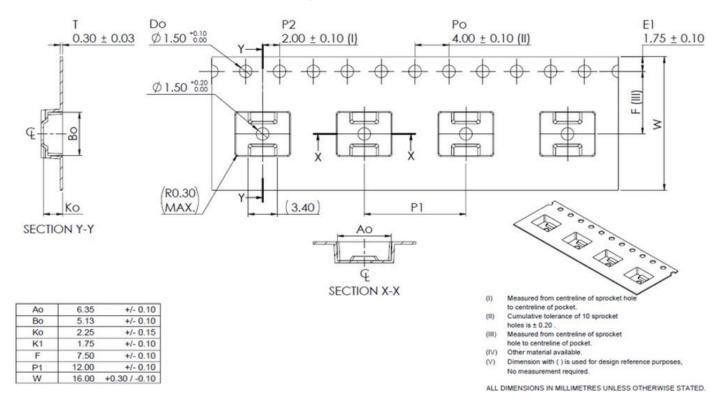
Figure 20: Tape and Pocket Drawing for SOIC-8 Package
