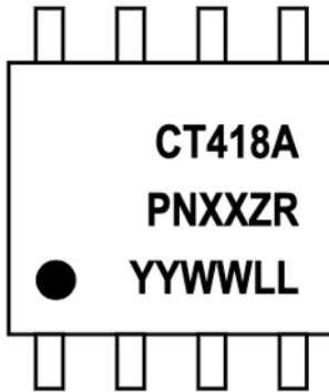
Figure 47: CT418 Device Marking for 8-lead Package
