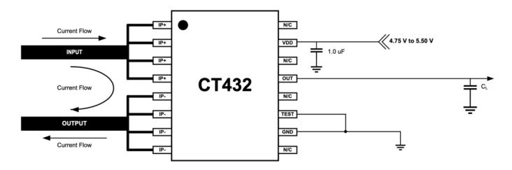
Figure 13: CT432 Application Block Diagram
