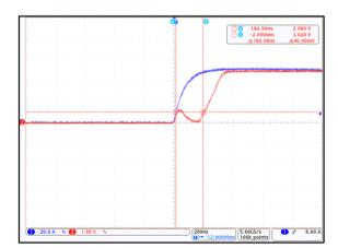
Figure 8: CT432 Propagation Delay;  $I_P = 50 A_{PK}$  and  $C_L = 100 pF$  (Blue =  $I_{CCC}$ , Red =  $V_{OUT}$ )
