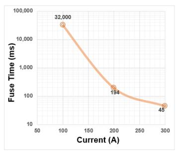
Figure 14: CT432 Fuse Time vs. Current
