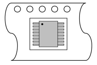
Figure 19: SOICW-16 Orientation in Tape Pocket
