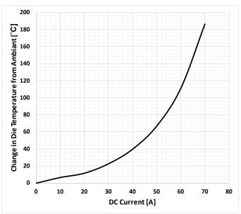
Figure 15: Self Heating in the LA Package Due to Current Flow
