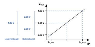
Figure 9: Linear Output Voltage Range (OUT) vs. Measured Current (IP)
