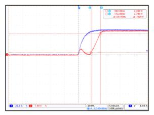
Figure 7: CT432 Rise Time;  $I_P = 50 A_{PK}$  and  $C_L = 100 pF$ (Blue =  $I_{CCC}$ , Red =  $V_{OUT}$ )
