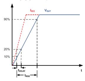
Figure 12: CT432 Propagation Delay and Rise Time Curve
