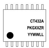
Table 3: CT432 Device Marking Definition for 16-lead SOICW Package
