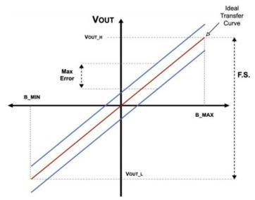
Figure 10: Total Output Error (E<sub>OUT</sub>) vs. Sensed Current (I<sub>P</sub>)
