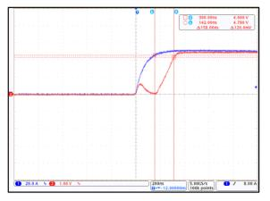
Figure 6: CT432 Response Time;  $I_P = 50 A_{PK}$  and  $C_L = 100 pF$  (Blue =  $I_{CCC}$ , Red =  $V_{OUT}$ )
