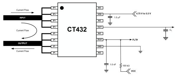
Figure 16: CT432 Application Block Diagram – With Overcurrent Detection
