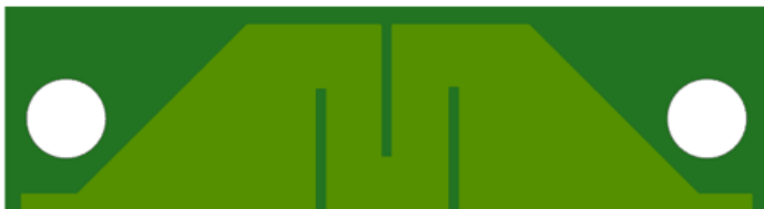
Figure 16: PCB Trace Design to Generate Differential Magnetic Field for CT452 to Measure
