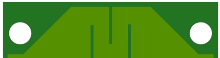
Figure 19: PCB Trace Design to Generate Differential Magnetic Field for CT452 to Measure
