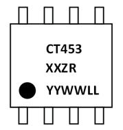
Figure 31: CT453 Device Marking for 8-Lead SOIC Package
