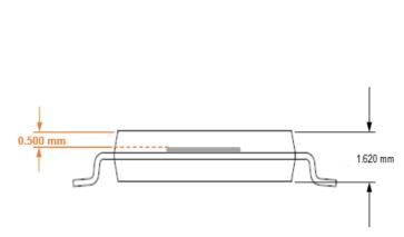
Figure 24: XtremeSense TMR Current Sensor Location in z Dimension for CT453 in SOIC-8 Package
