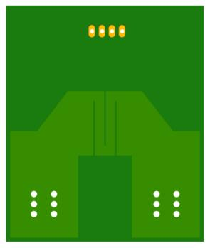
Figure 22: Recommended PCB Layout (Bottom Layer) for CT453
