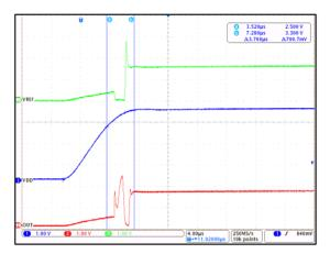
Figure 10: CT453 Startup Waveforms for V<sub>OQ</sub> = 1.65 V (Bipolar Field)
