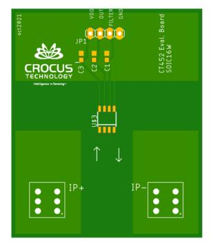
Figure 21: Recommended PCB Layout (Top Layer) for CT453
