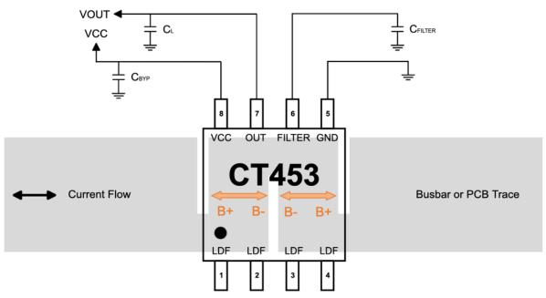
Figure 3: CT453 Application Diagram for SOIC-8
