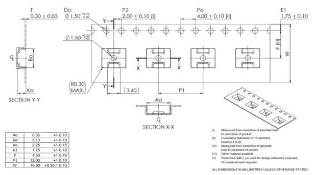
Figure 29: Tape and Pocket Drawing for SOIC-8 Package
