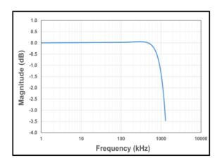
Figure 8: CT453 Bandwidth with C<sub>FILTER</sub> = 1.0 pF
