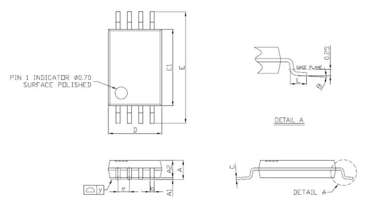
Figure 28: TSSOP-8 Package Drawing and Dimensions
