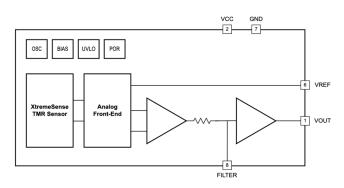
Figure 2: CT453 Functional Block Diagram for TSSOP-8
