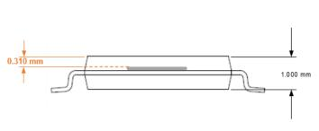
Figure 26: XtremeSense TMR Current Sensor Location in z Dimension for CT453 in TSSOP-8 Package
