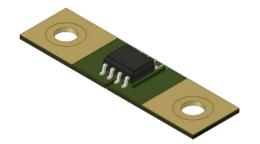
Figure 15: 3D View of CT453 and PCB Trace Design
