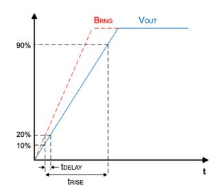
Figure 20: CT453 Propagation Delay and Rise Time Curve
