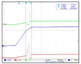
Figure 9: CT453 Startup Waveforms for V<sub>OQ</sub> = 0.65 V (Unipolar Field)
