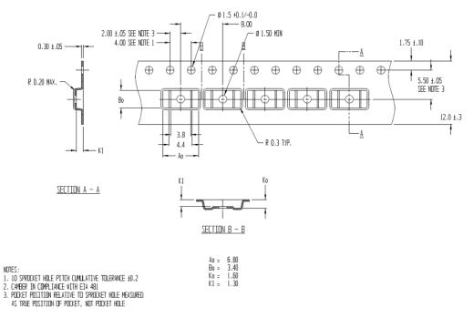
Figure 30: Tape and Pocket Drawing for TSSOP-8 Package
