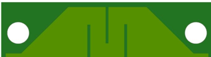
**Figure 16: PCB Trace Design to Generate Differential Magnetic Field for CT453 to Measure**
