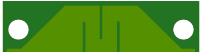
Figure 19: PCB Trace Design to Generate Differential Magnetic Field for CT453 to Measure
