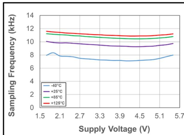
Figure 17: Sampling Frequency vs. Supply Voltage vs. Temperature
