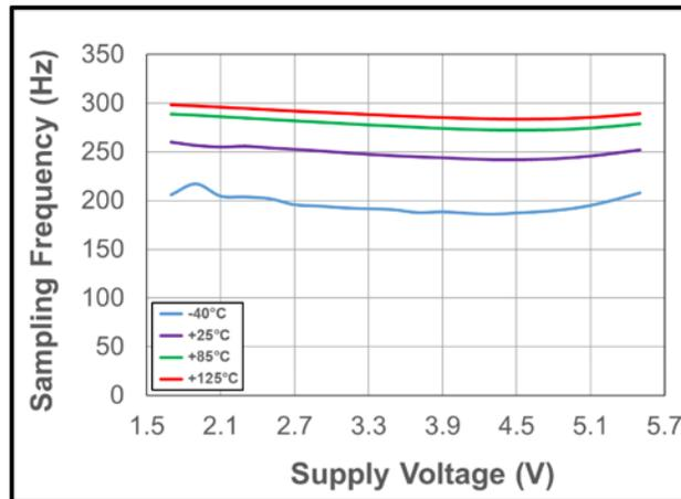
Figure 20: Sampling Frequency vs. Supply Voltage vs. Temperature
