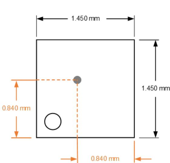
Figure 49: XtremeSense TMR Sensor Location for CT813x products in 3-lead SOT23 Package
