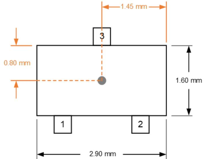
Figure 50: XtremeSense TMR Sensor Location for CT813x products in 4-lead LGA Package
