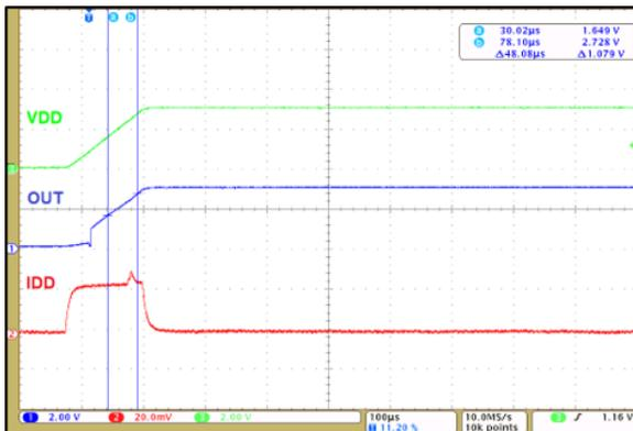
Figure 6: Power-On Time for Push-Pull Output
