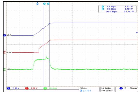
Figure 7: Power-On Time for Open Drain Output
