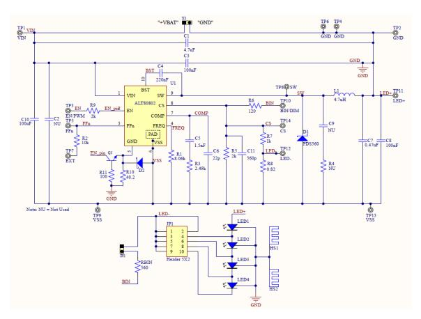
Figure 3: ALT80802 Evaluation Board Schematic
