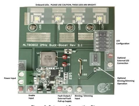
Figure 2: Setup and Connection Diagram
