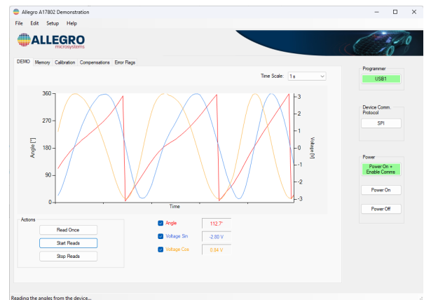
Figure 3: A17802/3 Allegro Application Samples Programmer (AASP)
