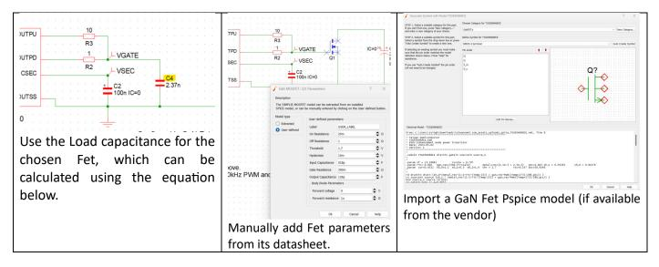
The FET used in the test bench is GS-66516-B from GaN Systems. From the GaN datasheet, the  $Q_{G(TOT)}$  is specified at 14.2 nC at 6 V VGS swing.
