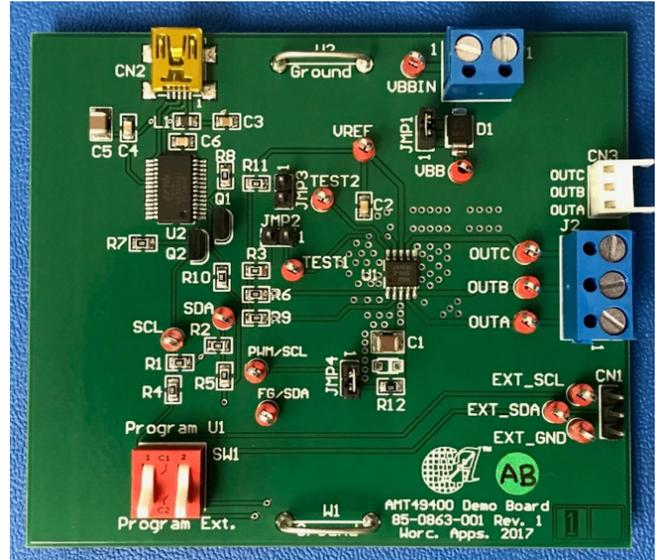
Figure 1: AMT49400 Evaluation Board
