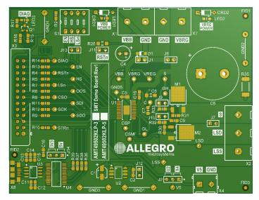
Figure 1: AMT49502 Evaluation Board
