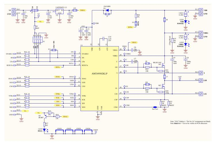
Figure 2: AMT49502KLP SMT Evaluation Board Schematic (1 of 2)
