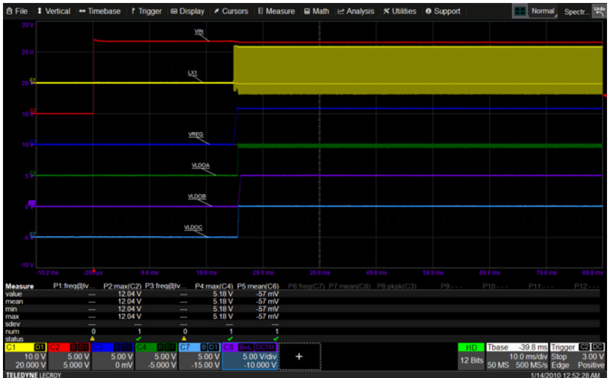
Figure 3: Startup Sequence Triggered on VIN
