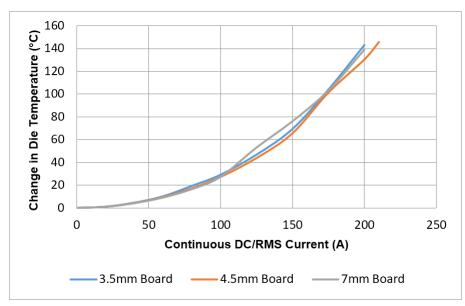
Figure 7: Continuous Current vs. Change in Die Temperature
