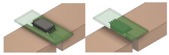
Figure 14: Application Assemblies (normal on the left, inverted on the right)
