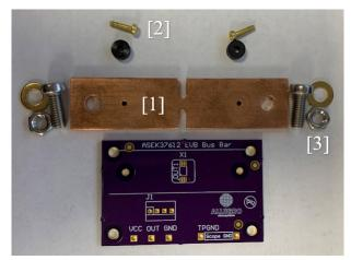
Figure 6: Printed Evaluation Board with Reference Busbar
