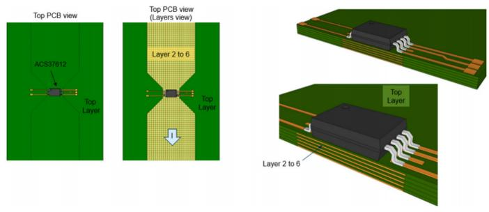
Figure 24: PCB Current Sensing Application
