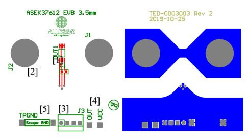
Figure 25: ASEK37612 EVB 3.5 mm PCB Top (left) and Bottom Layers (right)
