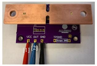
Figure 18: Sensor Connections
