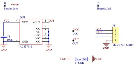
Figure 27: ASEK37612 EVB Schematic, 3.5 mm
