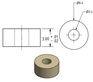
Figure 10: 3 mm Spacer
