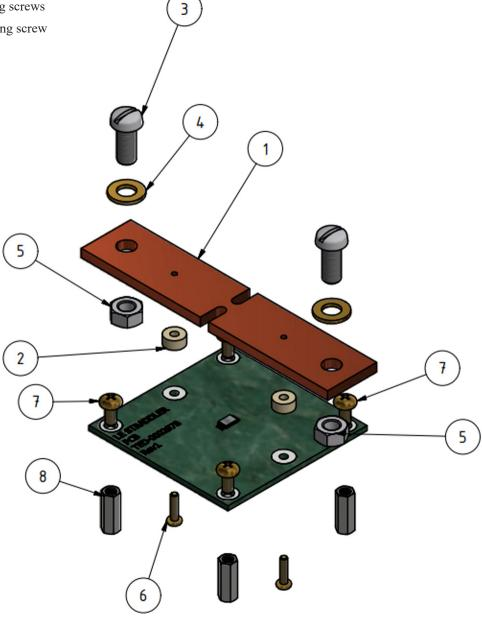
Figure 4: Exploded View of ASEK37612 Evaluation Kit Components
