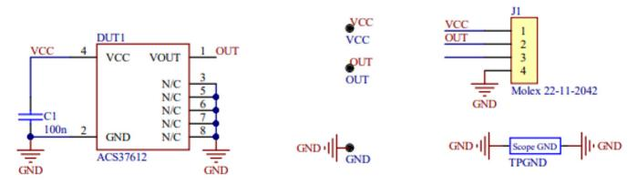
Figure 11: ASEK37612 Evaluation Board Schematic
