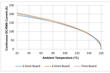
Figure 8: Ambient Temperature vs. Continuous Current
