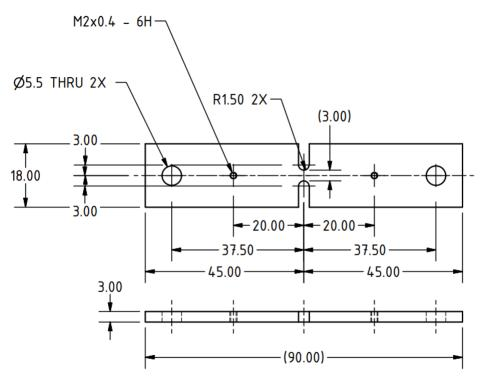
Figure 9: Reference Busbar Dimensions
