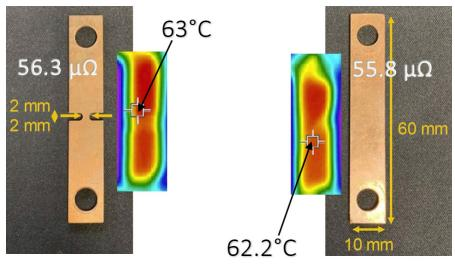
Figure 17: Thermal Comparison of Notched and Solid Busbar
