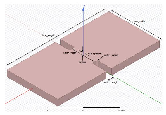
Figure 20: Reference Busbar Dimension Definitions
