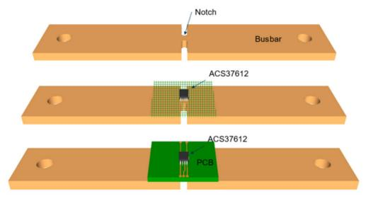
Figure 16: Busbar Current Sensing Reference Design
