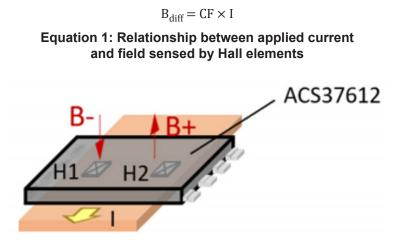
Figure 12: ASEK37612 Busbar and ACS37612 Hall Elements with Sensed Fields
