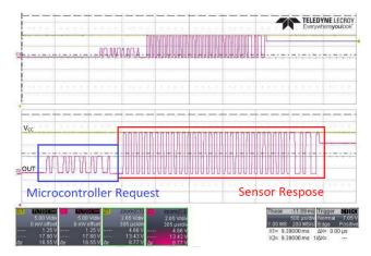
Figure 18: Oscilloscope capture showing the Manchester programming protocol on the output of the part
