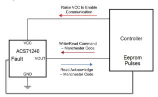
Figure 17: ACS71240 Programming Diagram
