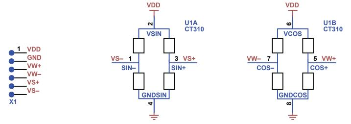
Figure 4: CT310 Evaluation Board Schematic
