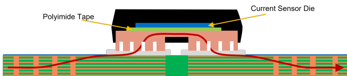
Figure 5: No Vias Under Copper Pads Example
