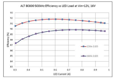
Figure 3: Efficiency vs Load
