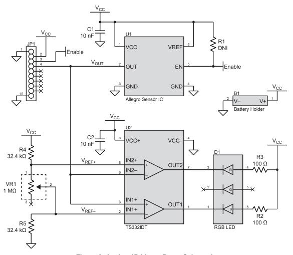
Figure 2: Analog 1D Linear Demo Schematic
