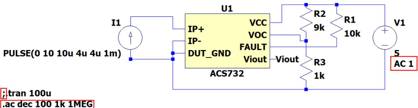
4. Right click on a blank portion of the schematic and again select “Run”. The simulation window will appear. To view the frequency response of the sensor output, hover over the Viout pin and click the
