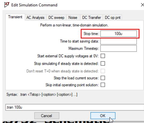
4. The transient simulation command will appear in the bottom left of the window.
