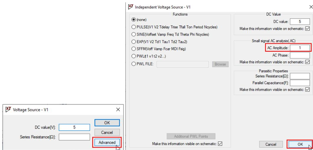
2. Ensure all other components pins of the symbol are given values. If an analysis has already been run, take the steps below. If no simulation has been run, right click on a blank portion of the schematic and select “Run”. This will open the “Edit Simulation Command” dialogue window where the user can chose and customize the desired simulation.
