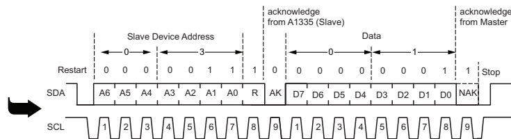
Figure 15: I 2 C Extended Address Write Example
