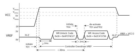
Figure 5: Communications Initialization Sequence with ANALOG\_LOCK = 1, UNLOCK\_CODE = 1
