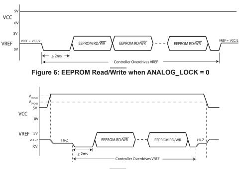
Figure 7: EEPROM Read/Write when ANALOG\_LOCK = 1
