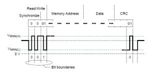
Figure 2: General Format for Serial Interface Communication
