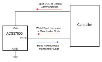
**Figure 1: Programming Connections**
