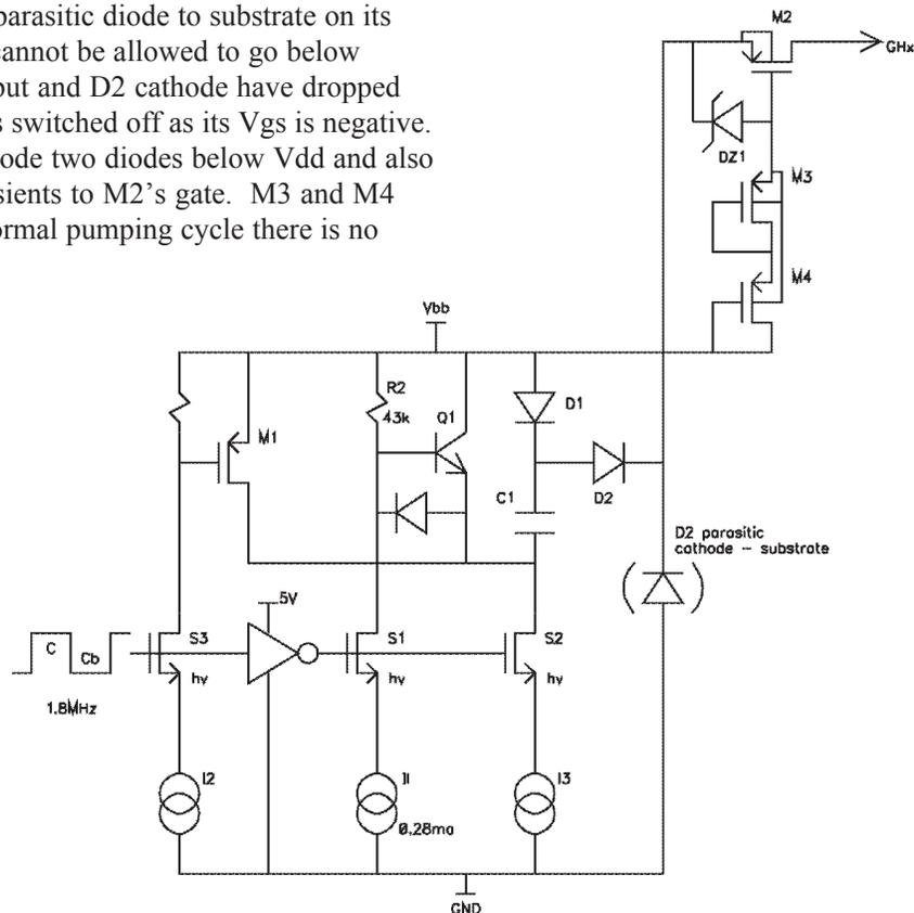
Figure 6 – Top-up charge pump
