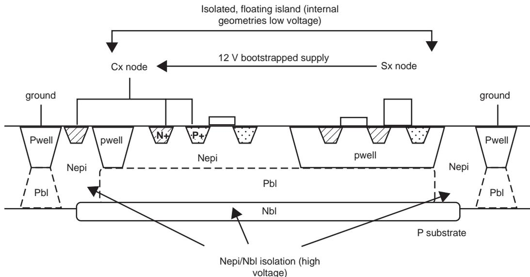
Figure 5 – High-side drive circuitry, isolated island structure
