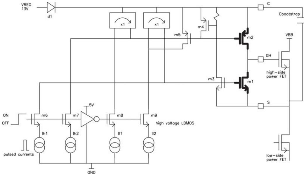
Figure 4 – High-side gate driver circuit
