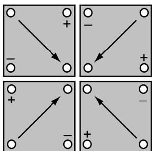
Fig. 21a. Four-element Hall device (arrows indicate current)
