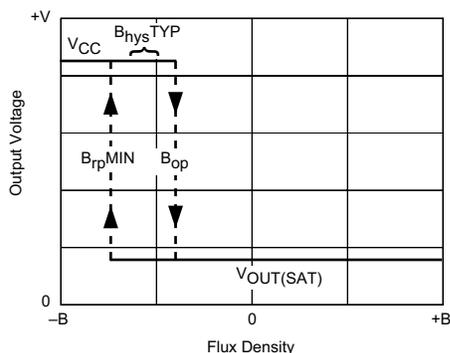
Fig. 9. Bipolar latch, negative unipolar mode
