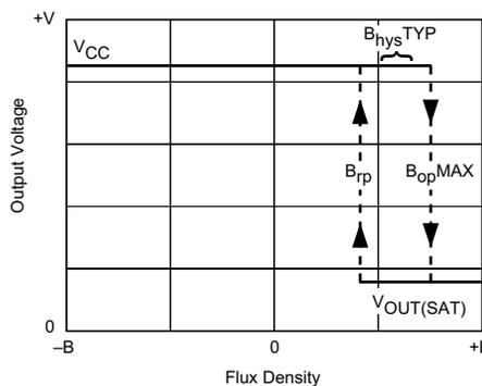
**Fig. 6. Unipolar switch or bipolar switch in unipolar mode**
