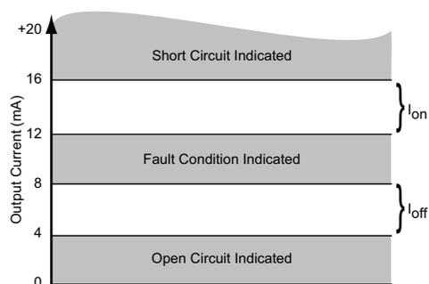
Fig. 12. Inherent fault detection (two-wire)
