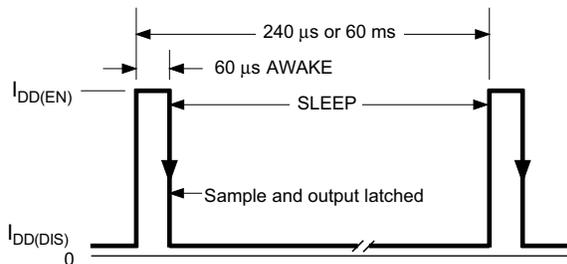
Fig. 23. Sleep mode to reduce current required
