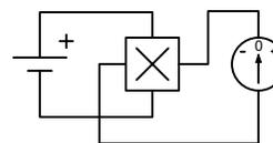
Fig. 2. Basic Hall device circuit
