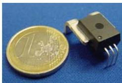
Fig. 19a. Hall current sensor IC
