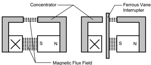
*Fig. 16. The right panel shows the vane shunting the magnetic field*
