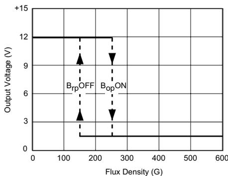
Fig. 11a. Voltage mode (three-wire)
