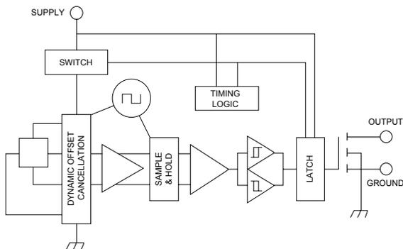
Fig. 24. Chopper-stabilized Hall circuit
