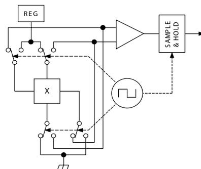
Fig. 22a. Chopper-stabilized Hall circuit
