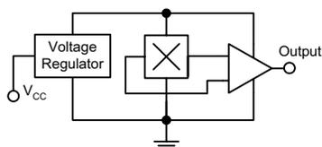
**Fig. 4. Circuit building block with signal augmentation circuitry**
