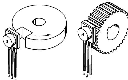
*Fig. 18. Proximity and gear tooth sensing*
