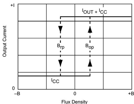
Fig. 11b. Current mode (two-wire)
