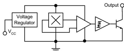
**Fig. 5. Practical Hall effect switch circuit**
