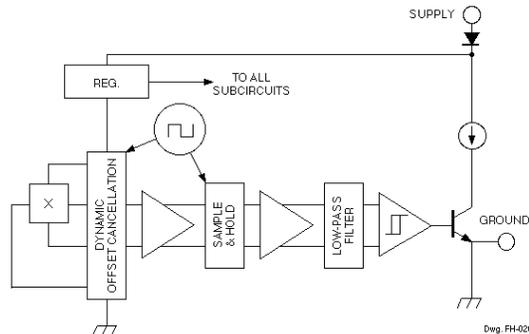
Fig. 10b. Two-wire configuration
