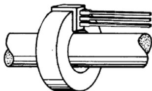
Fig. 19b. Use of split gap toroid for sensing higher current levels
