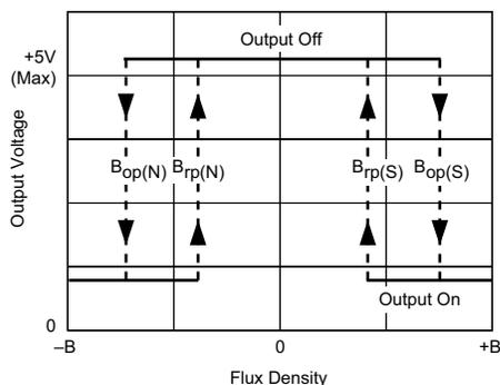
Fig. 7. Omnipolar switch. *N*, relative to north pole; *S*, relative to south pole.
