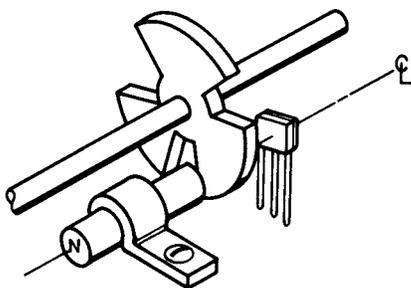
*Fig. 17a. Axle-mount vane interrupter*
