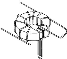
Fig. 19c. Use of multiple windings to increase flux density for low current sensing
