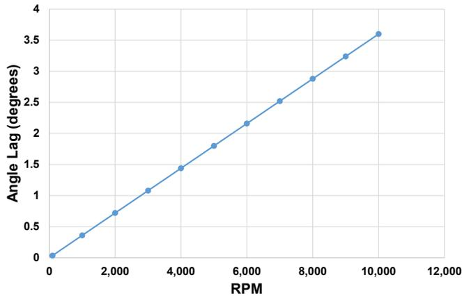
Figure 6: Angle Lag versus RPM, 60 µs Response Time
