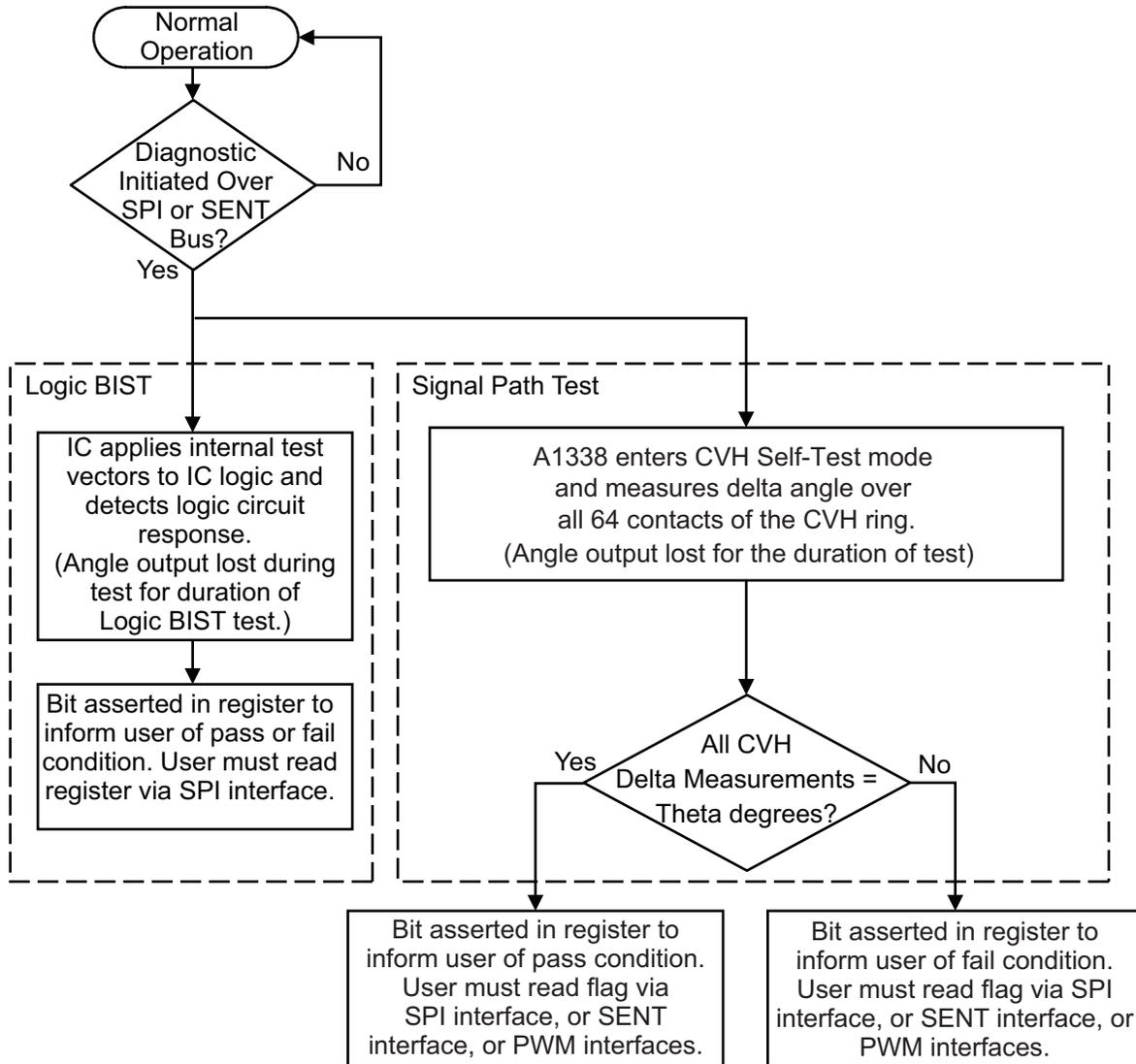
Figure 14: User-Interface Diagnostic Diagram
