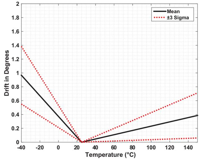
Figure 21: Angle Drift Relative to 25°C (300 G)
