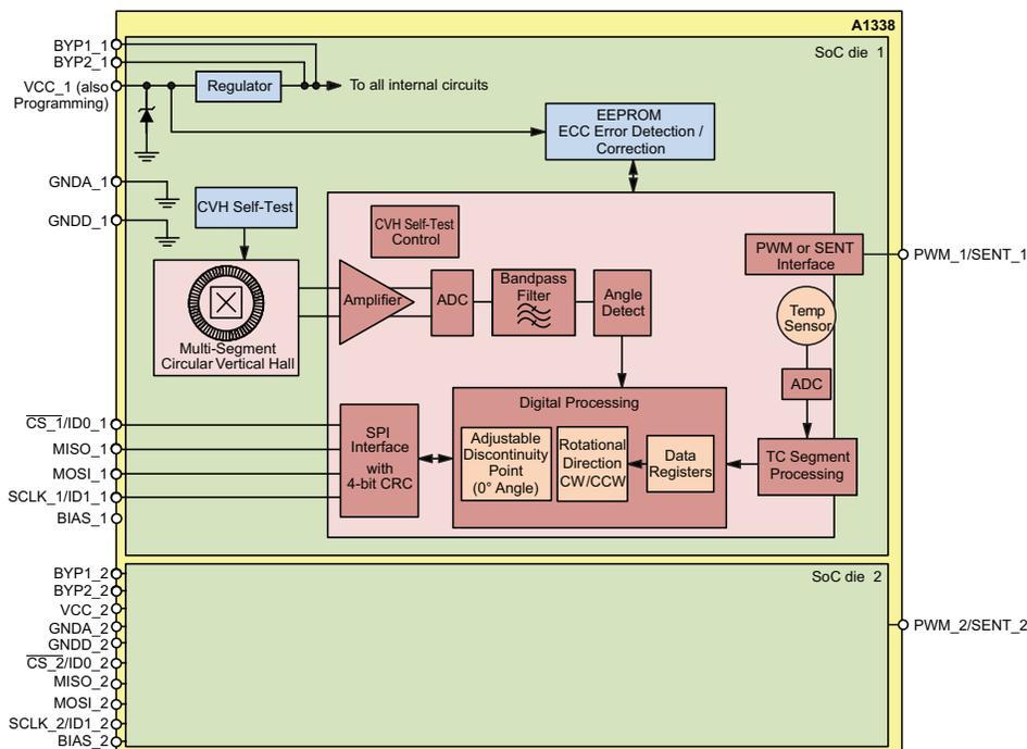
**Figure 1: A1338 Magnetic Circuit and IC Diagram**
