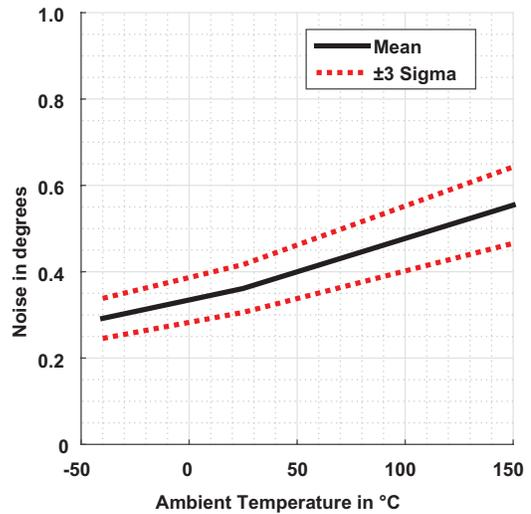
Figure 25: Noise Performance over Temperature (3  $\sigma$ , 300 G)
