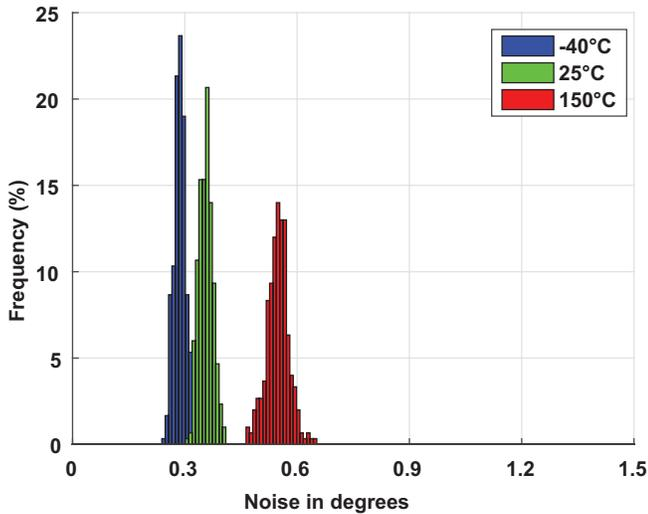
Figure 24: Noise Distribution over Temperature (3  $\sigma$ , 300 G)
