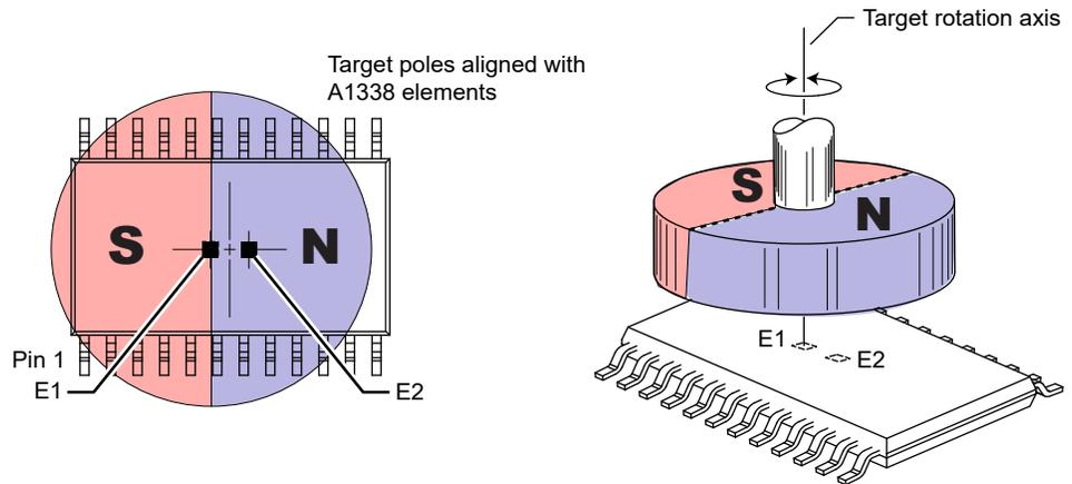
**Figure 15: Orientation of Magnet Relative to Die**
