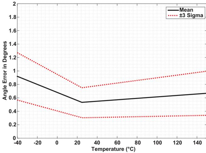
Figure 20: Angle Error over Temperature (300 G)
