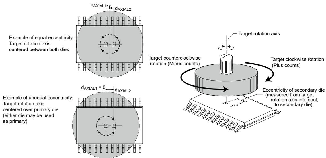
**Figure 19: Demonstration of Magnet to Sensing Element Eccentricity**
