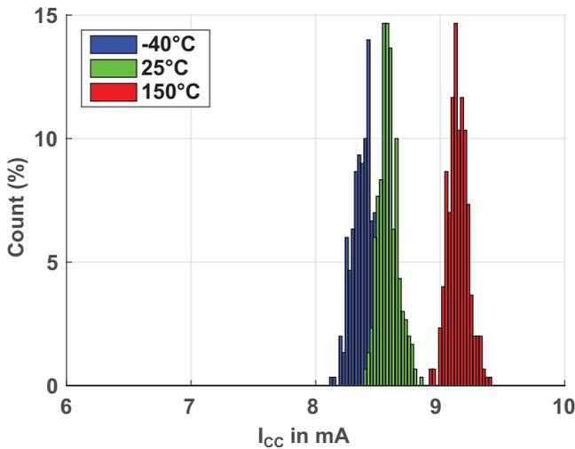
Figure 26:  $I_{CC}$  Distribution over Temperature ( $I_{CC}$ ,  $V_{CC} = 3.7$  V)
