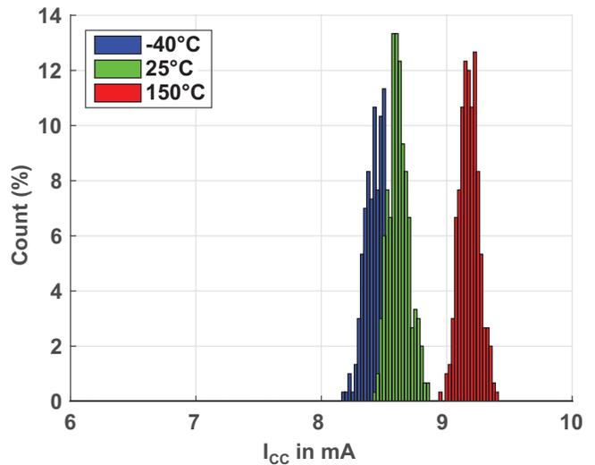
Figure 27:  $I_{CC}$  Distribution over Temperature ( $I_{CC}$ ,  $V_{CC} = 16$  V)
