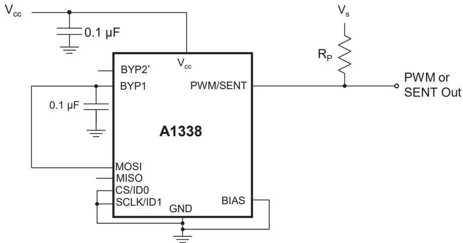
**Figure 3: Typical A1338 Configuration Using PWM or SENT Output. ID Value of 00<sub>2</sub>.**
