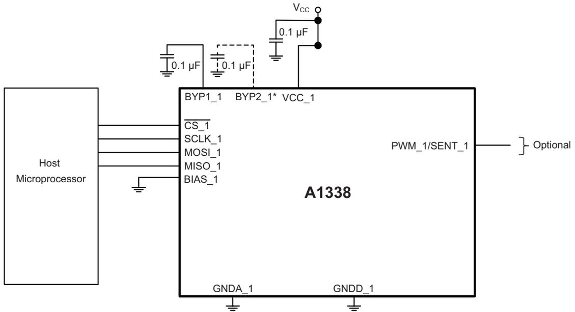
**Figure 2: Typical A1338 Configuration Using SPI Interface**
