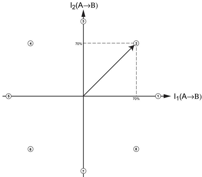
Figure 15: Half Step (70% Torque)
