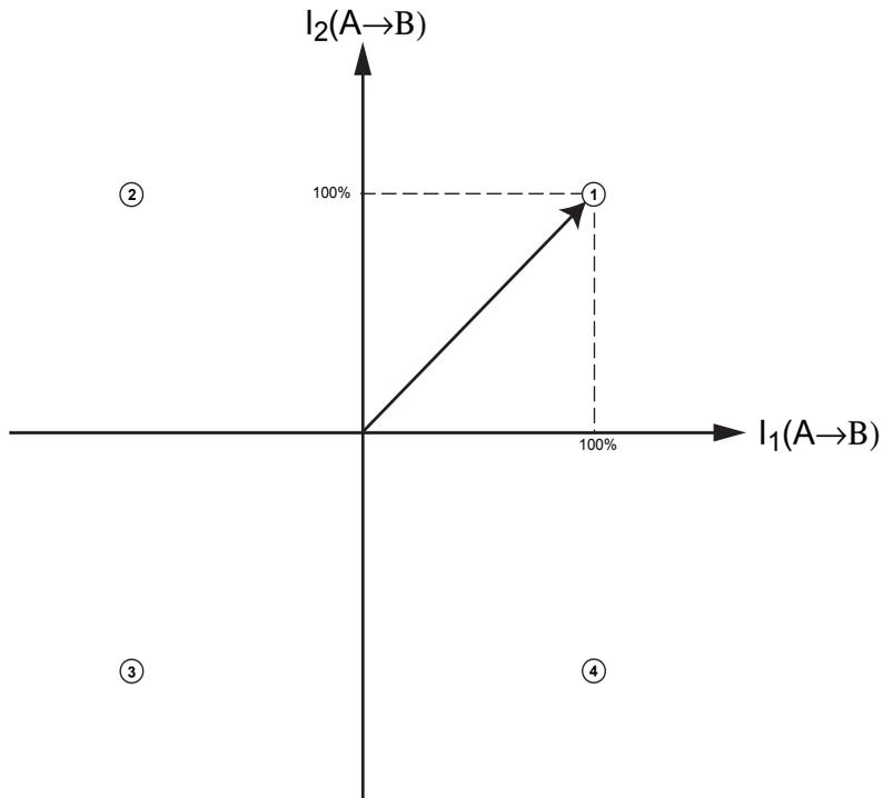
**Figure 10: Full Step (100% Torque)**
