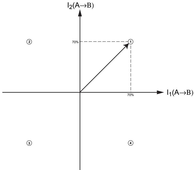
Figure 14: Full Step (70% Torque)
