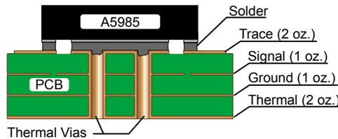
Figure 6: Soldering Cross-Section
