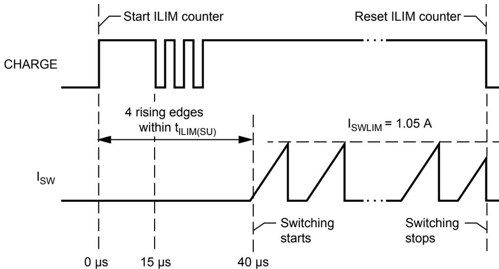
Figure 7. Current Limit Programming Example ( $I_{swlim4}$  selected)
