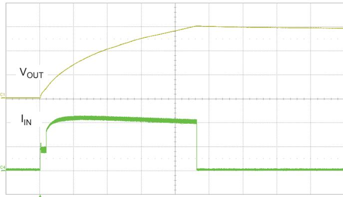
V<sub>BAT</sub> = 3.6 V. C1, V<sub>OUT</sub> 100 V/div, C4; I<sub>IN(av)</sub> 200 mA/div; Time 1s/div.
