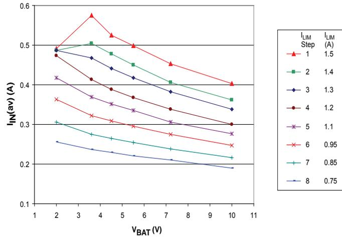
Note: Peak switch current is limited by maximum on-time and di/dt of transformer primary current; therefore, average current drops at very low battery voltage.
