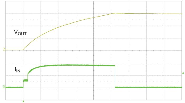
V<sub>BAT</sub> = 7.2 V. C1, V<sub>OUT</sub> 100 V/div; C4, I<sub>IN(av)</sub> 200 mA/div; Time 500 ms/div.
