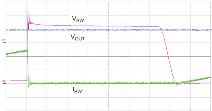
Figure 5. Zero-Voltage Switching (ZVS)  $V_{BAT} = 3.6$  V,  $I_{SWlim} = 1.2$  A. C2,  $V_{SW} = 2$  V/div; C3,  $V_{OUT} = 50$  V; C4,  $I_{SW} = 500$  mA/div; Time = 0.5  $\mu$ s/div.
