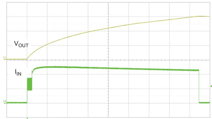
V<sub>BAT</sub> = 2 V. C1, V<sub>OUT</sub> 100 V/div; C4, I<sub>IN(av)</sub> 200 mA/div; Time 1s/div.
