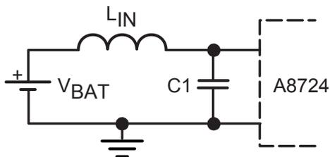
Figure 11. Typical input section with input inductance (inductance,  $L_{\text{IN}}$ , may be an input filter inductor or inductance due to long wires in test setup)
