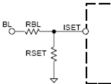
Figure 8. Optional Smart Current Limit configuration
