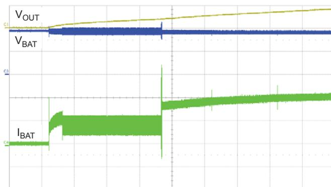
Figure 13. Input current waveforms with Li+ battery connected through 10  $\mu\text{H}$  inductor and 4.7  $\mu\text{F}$  capacitor. C1,  $V_{\text{OUT}}$  100 V/div; C3,  $V_{\text{BAT}}$  2 V/div; C4,  $I_{\text{BAT}}$  200 mA/div; Time, 50 ms/div.
