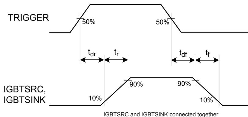
Figure 2. IGBT Drive Timing Definition
