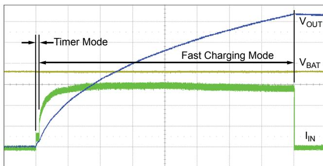
Figure 3. Timer mode and Fast Charging mode:  $t = 200$  ms/div;  $V_{OUT} = 50$  V/div;  $V_{BAT} = 1$  V/div.;  $I_{IN} = 100$  mA/div.,  $V_{BAT} = 3.6$  V;  $C_{OUT} = 20$   $\mu$ F/330 V; and  $I_{SWlim} \approx 0.75$  A.
