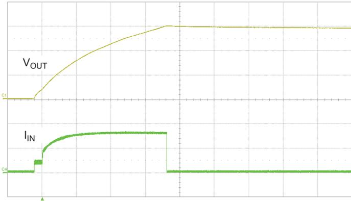
V<sub>BAT</sub> = 11 V. C1, V<sub>OUT</sub> 100 V/div; C4, I<sub>IN(av)</sub> 200 mA/div; Time 500 ms/div.
