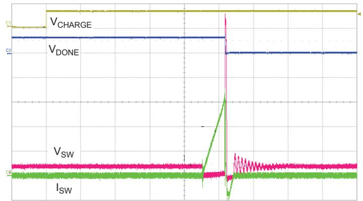
Figure 9. Operation under open diode fault ( $I_{SWlim} = 1.5$  A,  $V_{BAT} = 3.6$  V,  $L_{primary} = 12.8$   $\mu\text{H}$ ). C1,  $V_{CHARGE}$ , 5 V/div; C2,  $V_{SW}$  10 V/div; C3,  $\overline{DONE}$  5 V/div; C4,  $I_{SW}$  500 mA/div; Time, 10  $\mu\text{s}$ /div.
