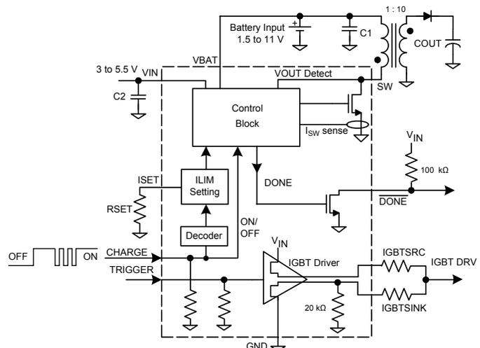
Figure 1b. Current programmed by CHARGE pin
