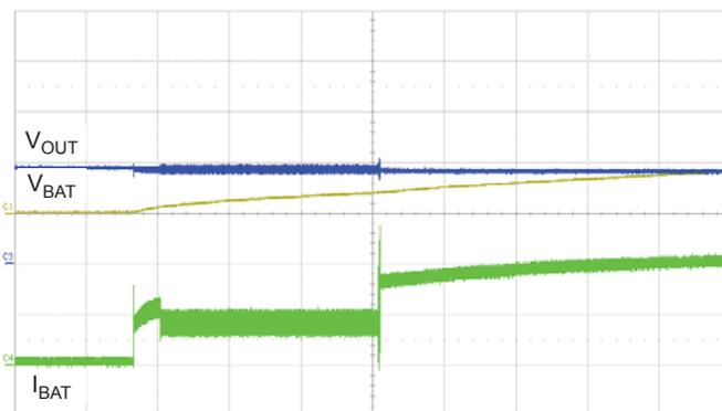
Figure 14. Input current waveforms with Li+ battery connected through 10  $\mu\text{H}$  inductor and 10  $\mu\text{F}$  capacitor. C1,  $V_{\text{OUT}}$  100 V/div; C3,  $V_{\text{BAT}}$  2 V/div; C4,  $I_{\text{BAT}}$  200 mA/div; Time, 50 ms/div.
