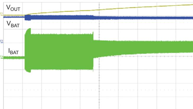
Figure 12. Input current waveforms with Li+ battery connected by 5-in. wire and decoupled by 4.7  $\mu\text{F}$  capacitor. C1,  $V_{\text{OUT}}$  100 V/div; C3,  $V_{\text{BAT}}$  2 V/div; C4,  $I_{\text{BAT}}$  500 mA/div; Time, 50 ms/div.
