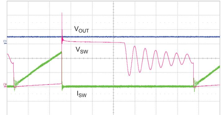
Figure 4. Expanded view of Timer Mode,  $V_{BAT} = 3.6$  V,  $I_{SWlim} = 1.2$  A. C2,  $V_{SW} = 2$  V/div; C3,  $V_{OUT} = 50$  V/div; C4,  $I_{SW} = 500$  mA/div; Time = 2  $\mu$ s/div.
