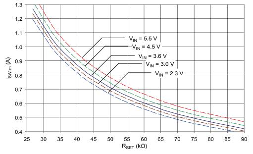
Figure 3. Peak Current Limit versus ISET Resistance.  $V_{IN} = V_{BAT}$ , transformer  $L_P = 8 \mu H$ ,  $T_A = 25^{\circ}C$ .
