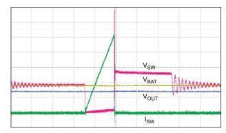
Figure 6. Timer Mode expanded view. V<sub>OUT</sub>  $\leq$  14 V, t = 2 µs / div., V<sub>BAT</sub> = 3.6 V, R<sub>SET</sub> = 33.2 kΩ.
