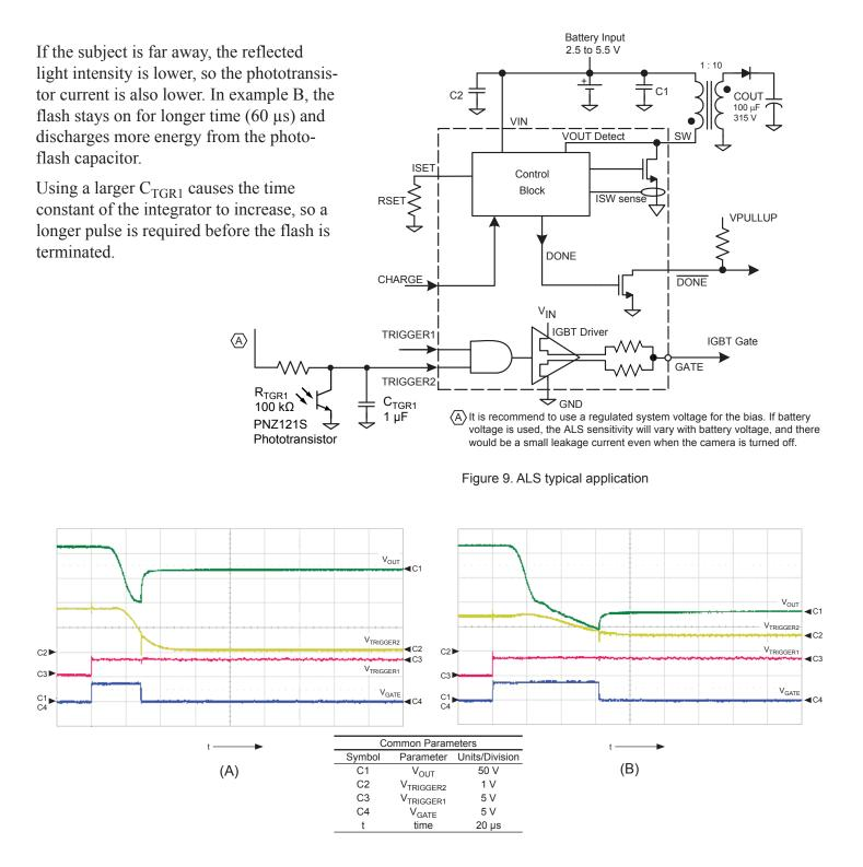
Figure 10. Adaptive timing of photoflash. (A) Subject near to camera, and (B) subject far from camera.
