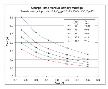
$C_{OUT}\text{=}~20~\mu\text{F}.$  For larger or smaller capacitances, charging time scales proportionally.
