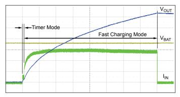
Figure 5. Timer Mode and Fast Charging Mode. t =200 ms/div, V<sub>OUT</sub> =50 V/div, V<sub>BAT</sub> =1 V/div., I<sub>IN</sub> =100 mA/div., V<sub>BAT</sub> =3.6 V, C<sub>OUT</sub> =20  $\mu$ F/330 V, R<sub>SET</sub>=46 k $\Omega$  (I<sub>SWlim</sub>≈0.75 A).
