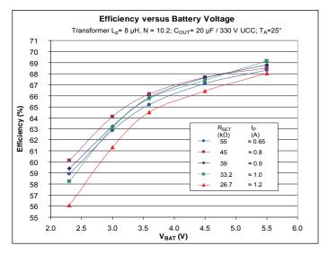
Special low-profile transformer with relatively low inductance (Lp= 8  $\mu$ H) and high winding resistance (Rp = 0.37  $\Omega$ ). Higher efficiency can be achieved by using transformers with higher Lp, which reduces switching frequency and therefore switching loses, and lower resistance, which reduces conduction losses.
