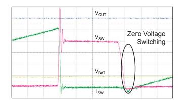
Figure 8. Zero voltage switching. V<sub>OUT</sub> = 120 V. t = 0.2  $\mu$ s/div., V<sub>BAT</sub> = 3.6 V, R<sub>SET</sub> = 33.2 k $\Omega$ .
