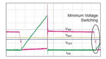
Figure 7. Minimum voltage switching. V<sub>OUT</sub>  $\geq$  15 V; t =1 µs/div., V<sub>BAT</sub> = 3.6 V, R<sub>SET</sub> = 33.2 kΩ.
