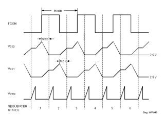
To avoid the capacitors charging to the supply rail, the value selected should provide adequate margin, taking into account the effects of capacitor tolerance, charging current, etc.
