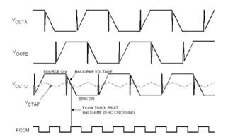
True back-EMF zero crossings are used by the adaptive commutation delay circuit to advance the state sequencer (commutate) at the proper time to synchronously run the motor. See next section.
