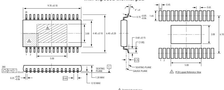
For reference only (reference JEDEC MO-153 AET) Dimensions in millimeters
