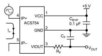
Application 1. The ACS754 outputs an analog signal,  $V_{OUT}$ . that varies linearly with the uni- or bi-directional AC or DC primary sampled current,  $I_P$ , within the range specified.  $C_F$  is recommended for noise management, with values that depend on the application.
