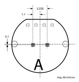
Lead Cross Section (in millimeters)
