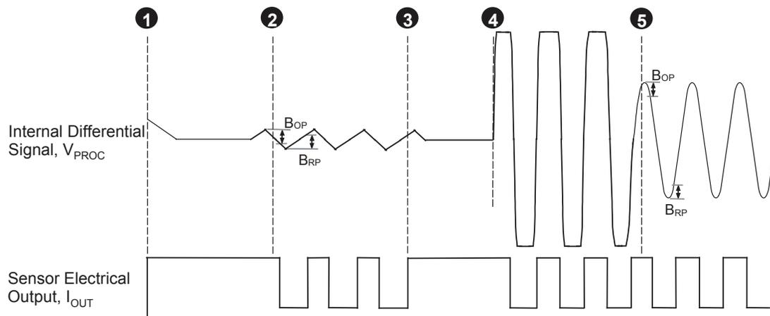
Figure 9: Operation of Running Mode Gain Adjust.
