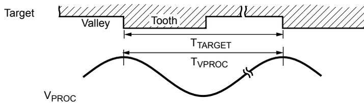
$V_{PROC}$  = the processed analog signal of the sinusoidal magnetic input (per channel)
