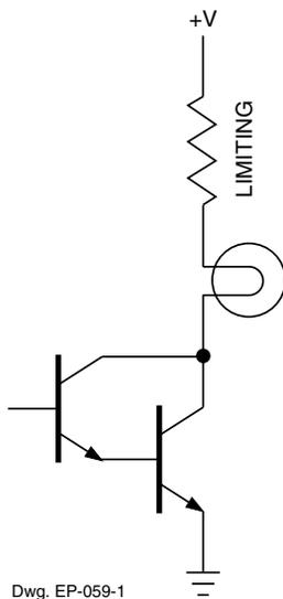
Figure 2 — Current-Limiting Resistor
