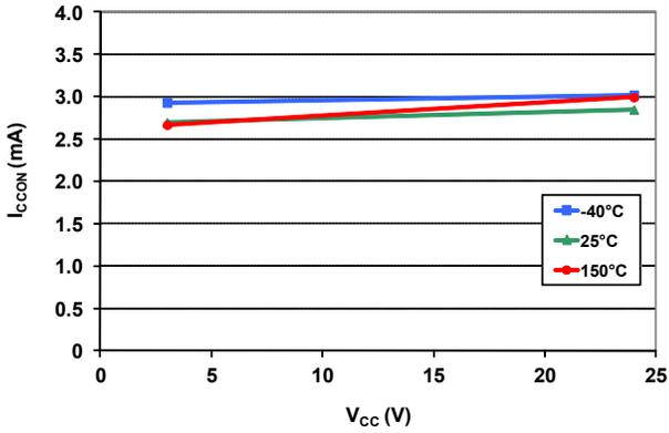
Supply Current (On) versus Ambient Temperature
