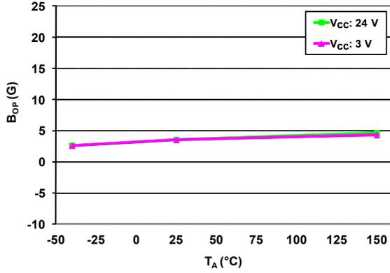
Release Point versus Ambient Temperature
