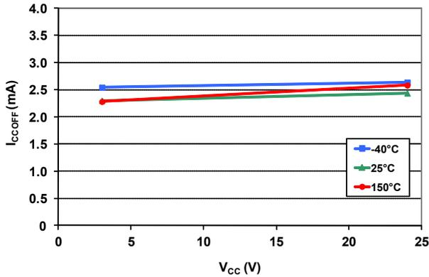
Supply Current (Off) versus Ambient Temperature
