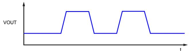
Figure 18: EEPROM Programming Pulses
