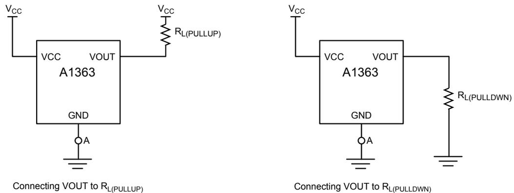
Figure 13: Connections for Detecting Broken Ground Wire
