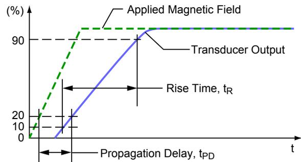
Figure 2: Propagation Delay and Rise Time Definitions
