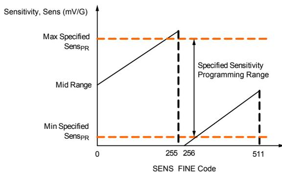
Figure 8. Device Sensitivity versus SENS\_FINE Programmed Value
