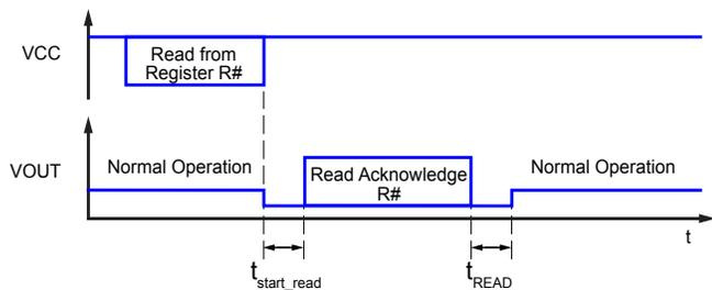
Figure 19: Reading from EEPROM or Volatile Memory
