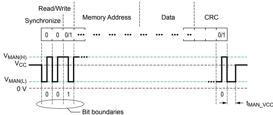
**Figure 22: V<sub>CC</sub> Levels During Manchester Communication**
