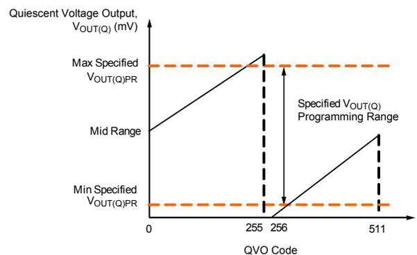
Figure 9. Device  $V_{OUT(Q)}$  versus QVO Programmed Value
