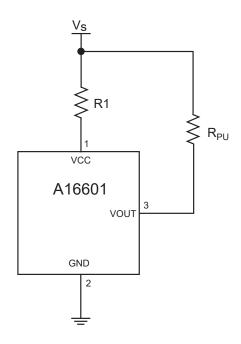
Figure 3: Recommended EMC Test Circuit
