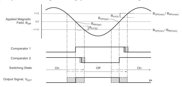
Figure 4: Typical output characteristics with dual comparator operation. Characteristics shown without delay; see Characteristic Data section charts for delay and phase shift contributions.
