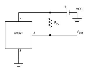
Figure 6: Basic application circuit. A pull-up resistor,  $R_{PU}$ , is required with the output driver.
