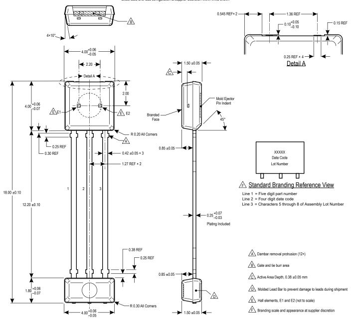
Figure 7: Package UC, 3-Pin SIP
