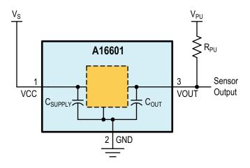
**Figure 2: Typical Application Circuit**
