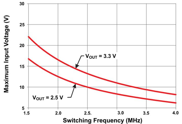
**Figure 3: Recommended Switching Frequency vs. Maximum Input Voltage**
