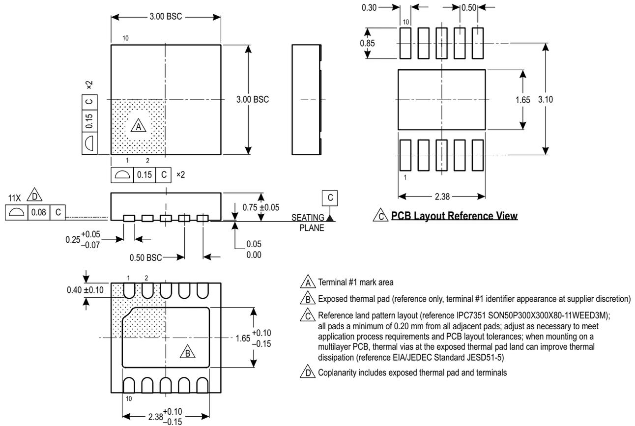
**Figure 7: Package EJ, 10-Pin DFN with Exposed Thermal Pad**
