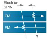
Figure 9: TMR Junction Showing Two Ferromagnets and a Tunnel Barrier
