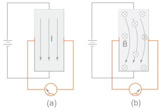
Figure 1: The Hall Effect in a Thin Plate
