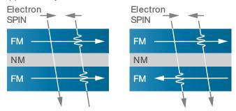
Figure 7: GMR Structures Showing Spin-Dependent Scattering
