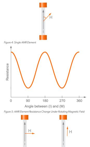
Low Resistance High Resistance Figure 6: Two AMR Elements Under Different Magnetic Fields
