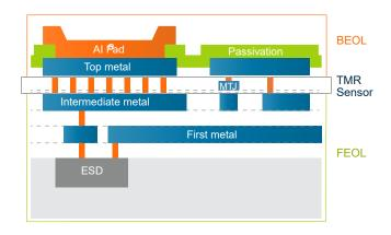
Figure 12: Typical CMOS Structure
