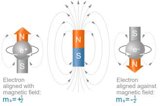
Figure 3: The Two Possible Spin Positions of an Electron
