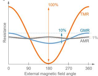
Figure 10: Signal Amplitude Comparison of AMR, GMR, and TMR (not to scale)
