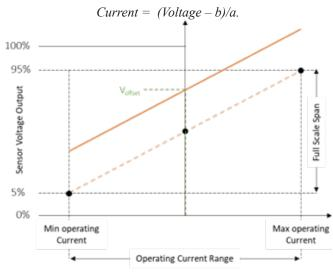
Figure 4: Simple Offset Calibration
