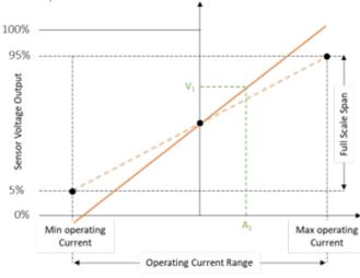
Figure 5: Simple Gain Calibration
