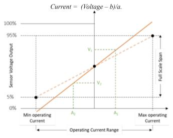
Figure 6: Gain Calibration
