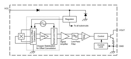
Figure 2. Modern Hall-effect sensor ICs integrate signal conditioning and amplification techniques to make practical devices.
