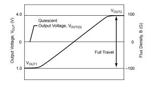
Figure 11. Example of the dynamic range for a linear Hall-effect IC.
