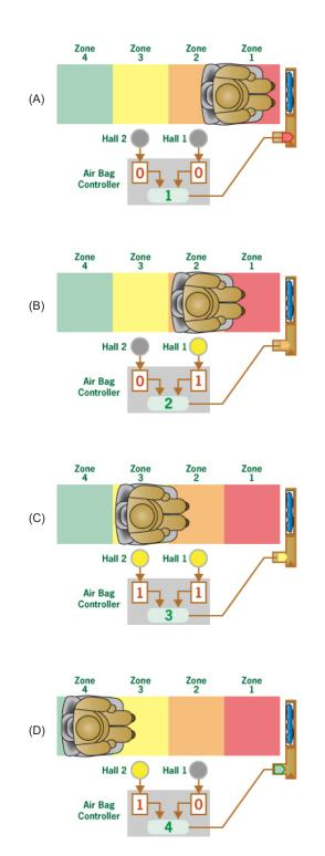
Figure 2. Position sensor ICs relay proper seat location to the controller unit the entire time the vehicle is on. Occupants are unaware of the fact that the vehicle is making life or death decisions automatically with no user interface required.
